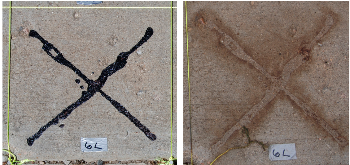
Figure 3: The image of grid 6L on the day the blood was deposited (a) compared with the same grid on day 5 (b) after having been rained on. This illustrates how the original stain was outlined by the diffusion of the stain into the surrounding concrete. A careful comparison will show that the outline is true to the original shape of the stain and retains many fine details.
