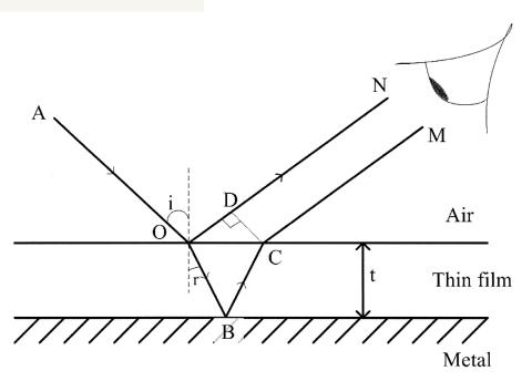
Figure 1: Optical interference in a thin film caused by an optical path difference between rays reflected and refracted at the airthin film surface.
