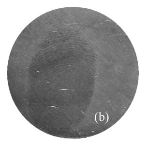
Figure 4: Fingerprint deposited on a brass disk heated subsequently to T = 250°C. (a) shows the disk before and (b) after digital color mapping.
