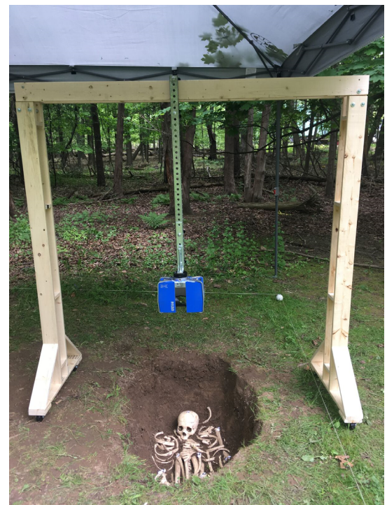
FIGURE 2: Wooden rig that was set up to invert the FARO laser scanner. This allowed for the scanner to be closer to the grave and the skeletal remains, eliminating the extra noise of the surrounding scene.
