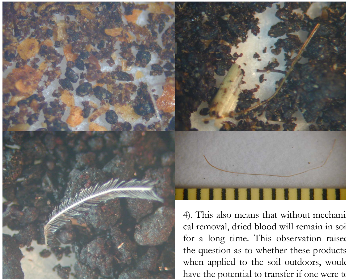
Figure 3: Microscopic appearance: Uncle Ians with 11% chili powder (upper left); 100% dried blood with bone (upper right); feather in the product (lower left); single hair recovered (lower right).
